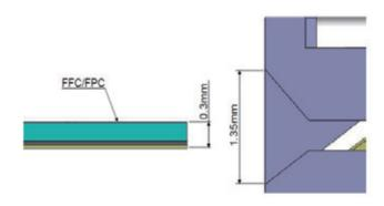
FPC / FFC insertion workability FPC / FFC has a thickness of 0.3 mm and guidance function (1.35 mm).
